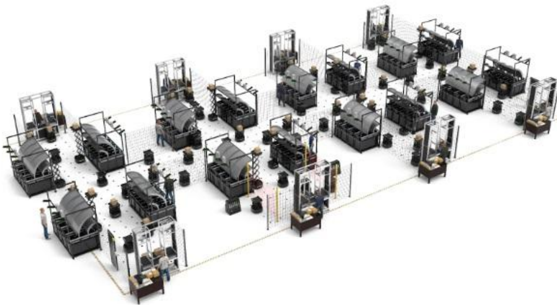
Unbox robotics mobile robots parcel sortation system “UnboxSort”
